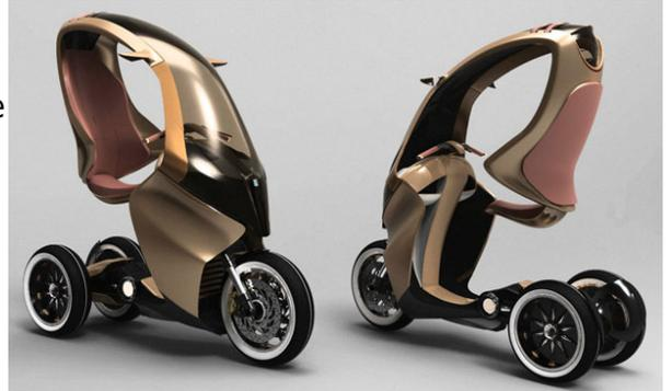
This new scooter was actually a student's thesis, carried out with the blessing of the Piaggio, the famous maker of Italian scooters. It features an lean-steering system; that is, all three wheels can pivot to let the whole scooter lean into a turn, which helps control and stability.
